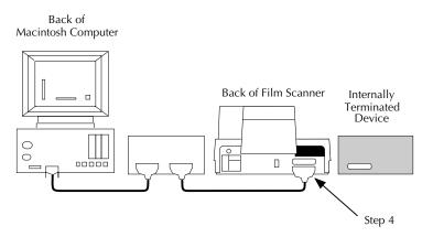
5. Attach the Scanner to the internally terminated device by plugging one end of your 50-pin to 50-pin SCSI cable into the empty SCSI port on the Scanner and the other end into the empty SCSI port on the terminated device. Seat both connectors firmly and pinch both wire clamps shut.
